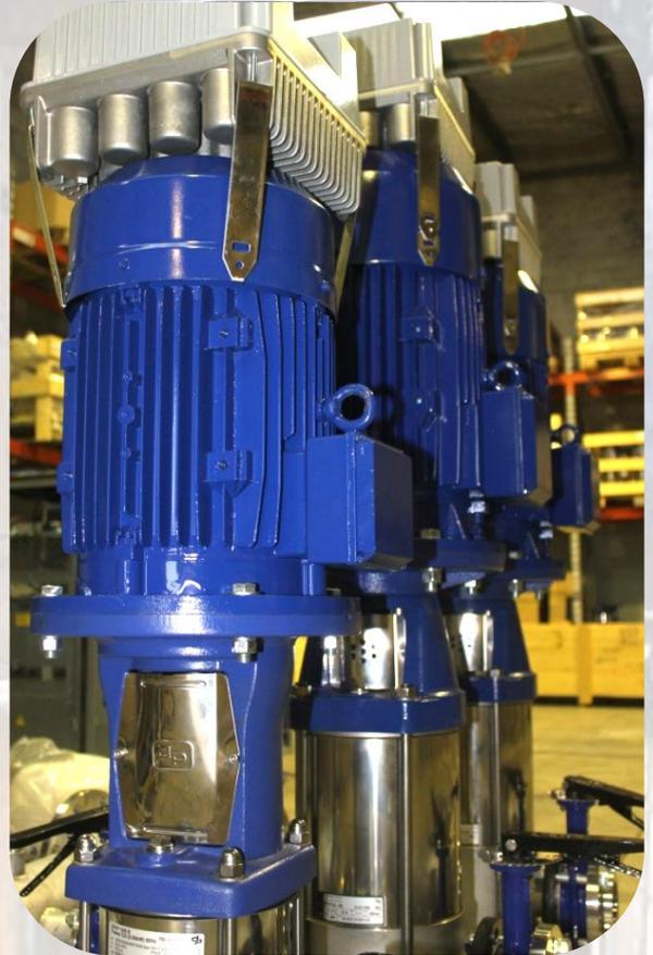
One major advantage of the Vasco motor mount VFD system is no load protection. This protects each pump units against dry running. An adjustable overload ts cannot detect if one pump is air locked, the Vasco VFD can pick this up as 'no load'. The operator is alerted by an audible and visual alarm. Audible and visual alarm can be muted.
